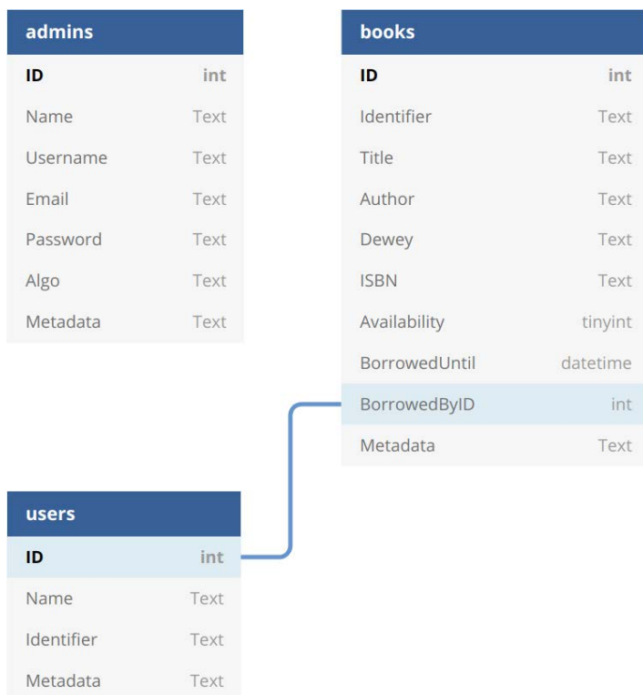
Image 10. SQL Database structure diagram
